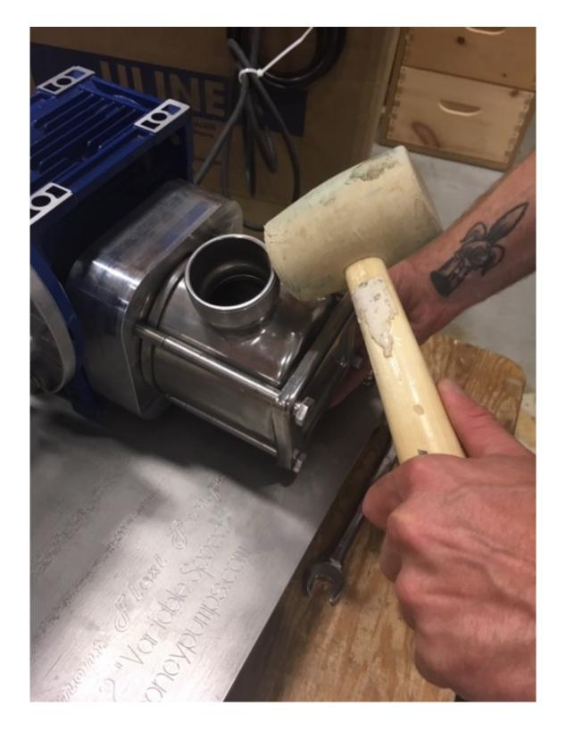
If it's difficult, you can use a soft hammer to push the housing in the lid while tightening the bolts.
