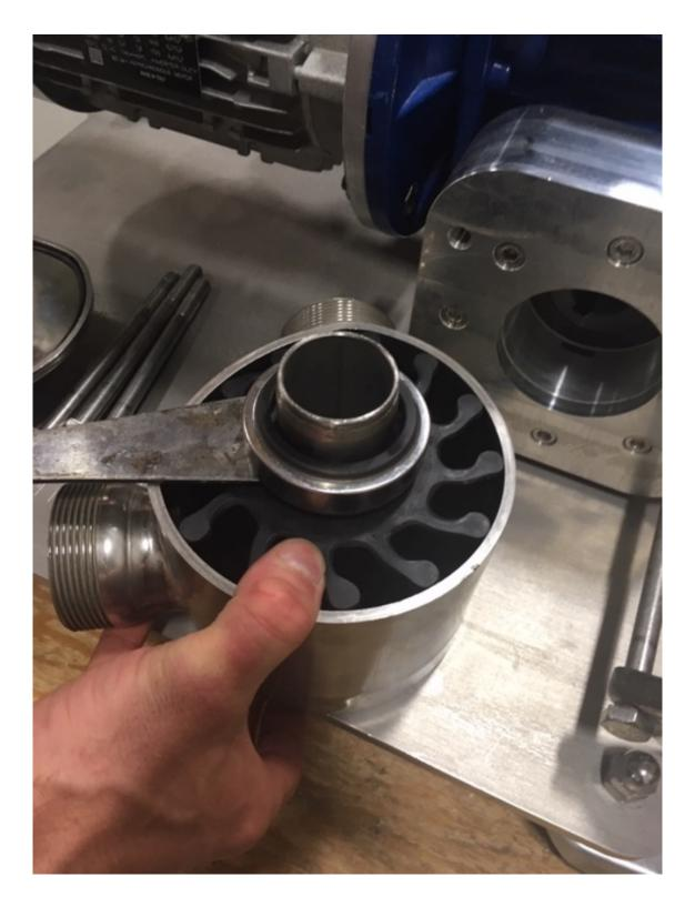
This part of the seal, if difficult, can be removed using a hive tool or a flat head screwdriver. Remove the old one and replace it with the new one.
