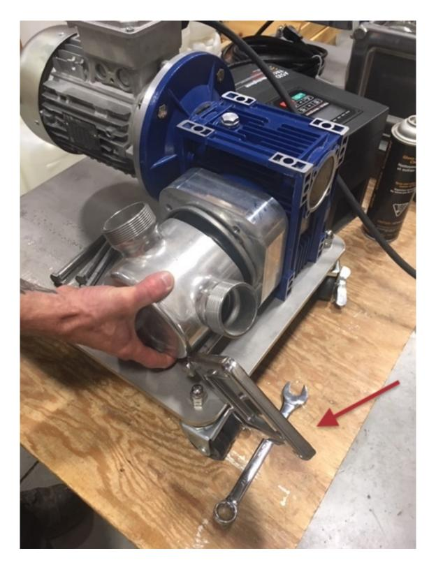
Move the plate aside and now the pump can be removed.
