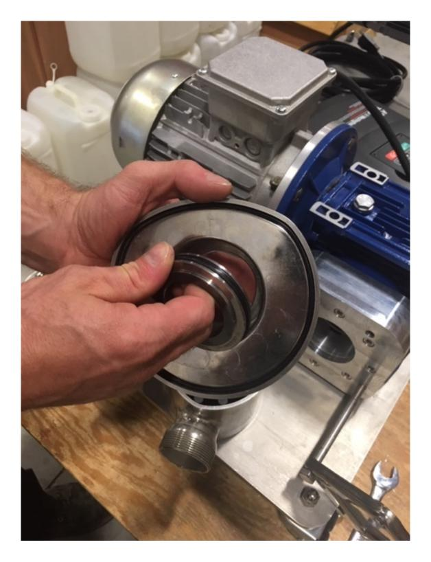
This part can be removed by hand. Take care while replacing the old one, push evenly and straight out. Use only your hands, do not use a hammer.
