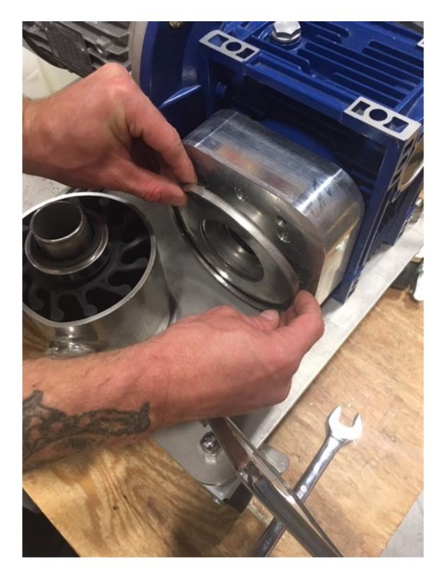
The pump has 4 parts; the housing, the lid, the impeller, and the seal.
