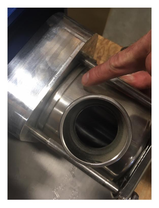
The housing must be well inserted in the lid.
