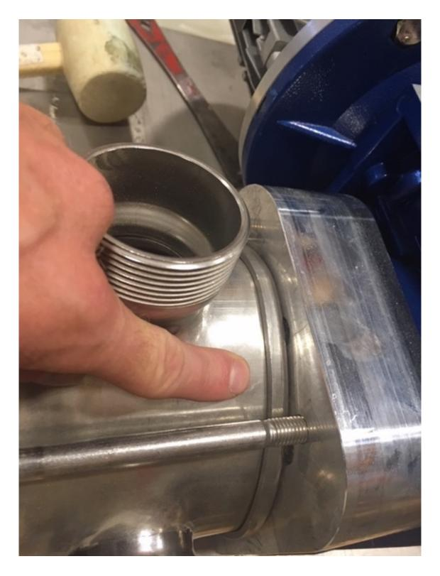
If a leak occurs, the housing is not well inserted in the lid, or the bolts are not tight enough.
