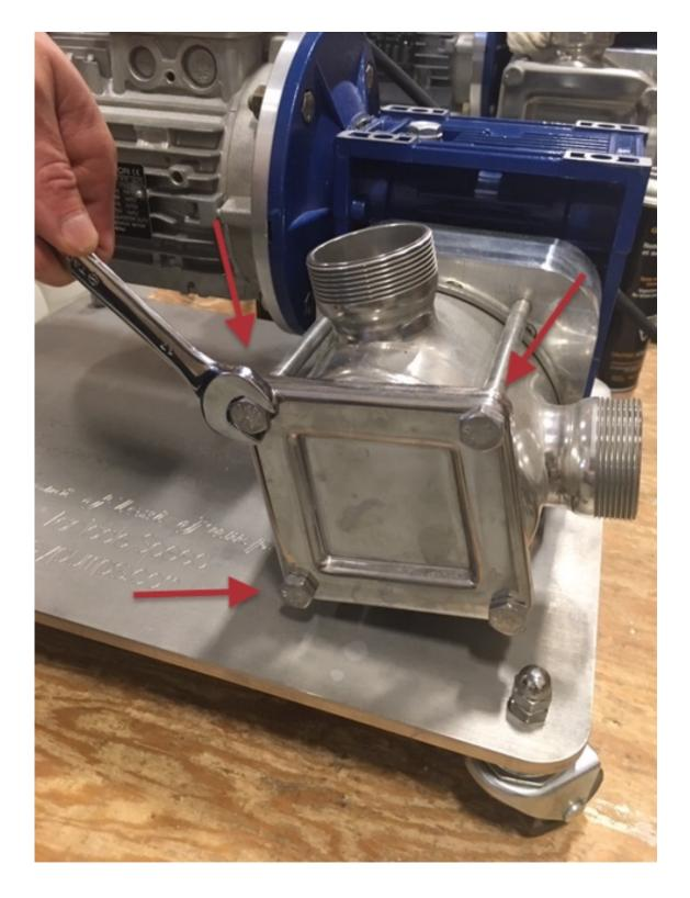
Remove only 3 bolts using a 17 wrench and loosen the 4<sup>th</sup>.
